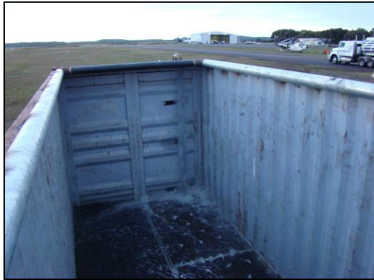
Image shows filling of the dip tank, sealant on the floor and around the doors and the cylindrical bump stop fitted to the rim.
